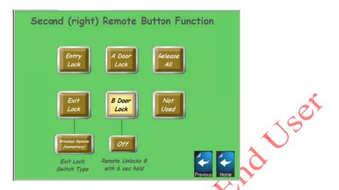
This screen is used when the Two Button Wireless Remote option is installed. It allows selection of the function controlled by the right button on the wireless remote control. The left button on the remote controls the reset of the metal detector alarm, and is a momentary pushbutton. The default setting for the second button is "B Door Lock"; any one of the other choices can be selected.
