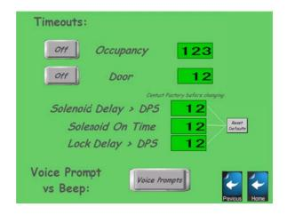
For systems equipped with the <u>bidirectional</u> door at the "B" location, all 3 values are available for setting the timing of the centering solenoid operation. "Reset Defaults" will change them back to the factory default values.
