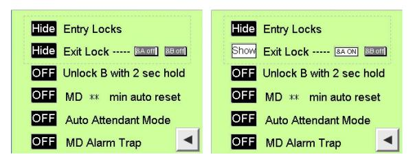
**Entry and Exit Locks**: Default settings are "Hide". The upper two selections allows the display of Lock Control Buttons on the Main screen. The Entry lock buttons allow locking the A or B doors independent of the system logic. The Exit lock allows trapping in the exit lane – the C door will open if the lane is unoccupied, but once someone enters the exit lane and C door closes, if the Exit Lock is on, the D door will not unlock. Touch the "Hide" to change to "Show".
