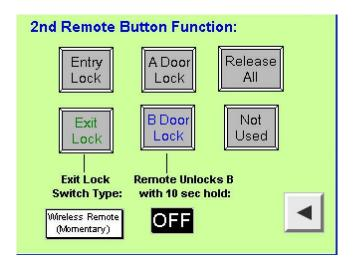
This screen is used when the "two button wireless remote" option is installed. It allows selection of the function controlled by the right button on the wireless remote control. The left button on the remote controls the reset of the metal detector alarm, and is a momentary pushbutton. The default setting for the second button is "B Door Lock"; any one of the other choices can be selected.
