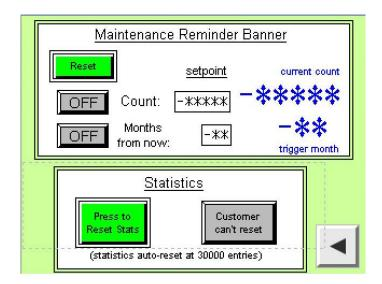
The Console has the option to display a banner along the bottom of the screen for maintenance reminder purposes. This is useful to remind your customer to make an appointment for preventive maintenance on a regular basis.
