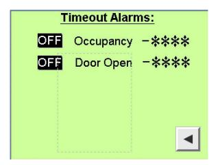
This screen allows enabling or disabling the occupancy and door open timeouts as well as changing the default values of the timeout times as desired. To change a timeout value, touch the value box to be changed, enter the new value on the keypad, and press the enter key. Default values are timeouts ON and set to 45 seconds (Occupancy) and 15 seconds (Door).
