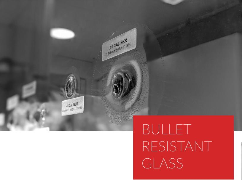
Anti-Attack glass comes standard in all Isotec units, although Bullet Resistant (BR) glass as high as UL Level 8 has been incorporated into systems. Our team will evaluate what level glass is required for the site.
